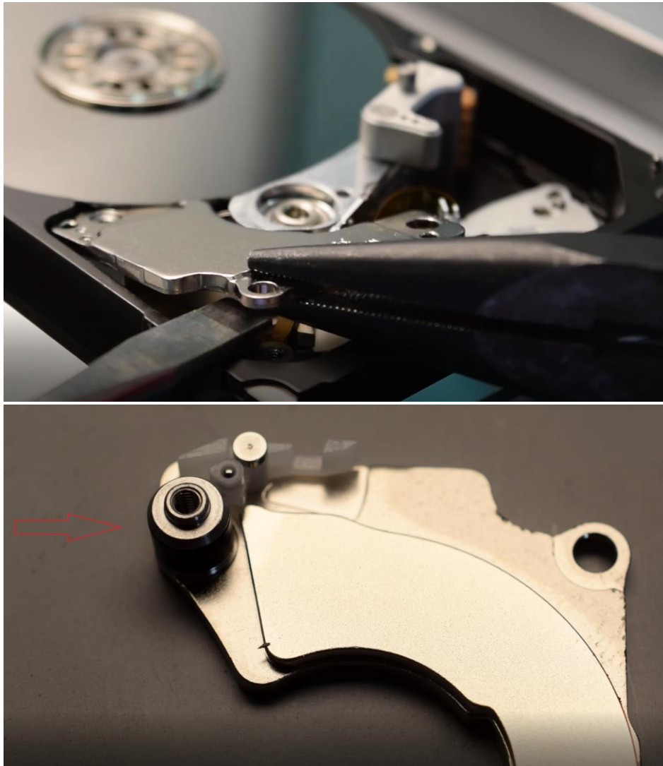
Picture 5.7. Dismounting the upper magnet
