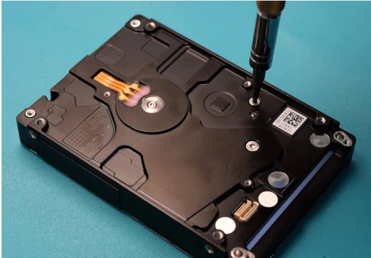
Picture 5.2. Removing the bottom screw
