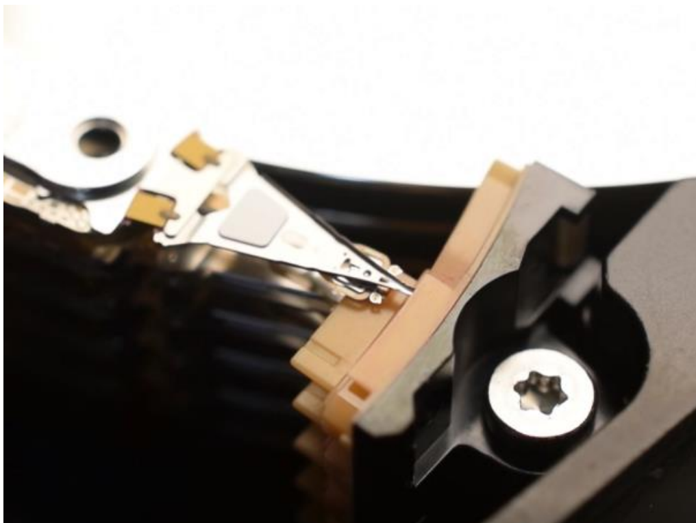
Picture 5.3. Moving the heads
