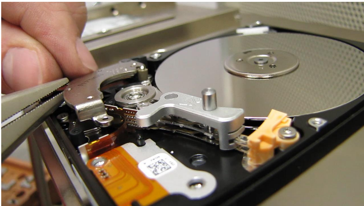
Picture 14. (moving the heads to the ramp)
