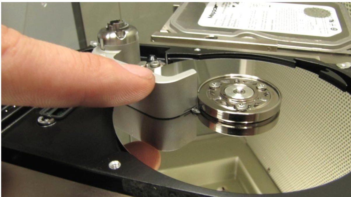
Picture 3. (Lifting the heads)
