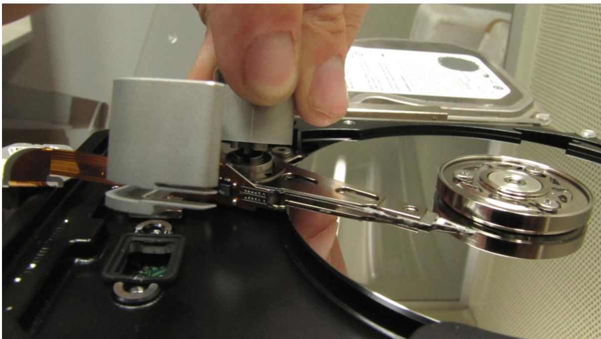
Picture 2. (Mounting the tool)
