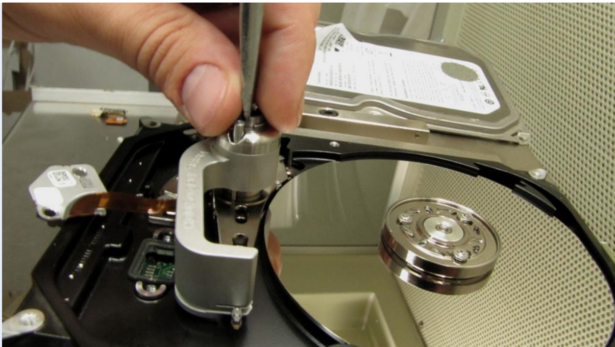
Picture 7. (Mounting the heads on a patient drive)
