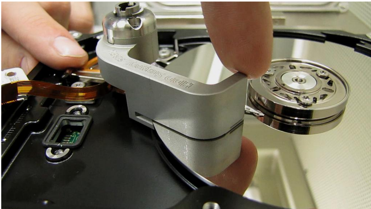
Picture 9. (Returning the tool outside of platters)
