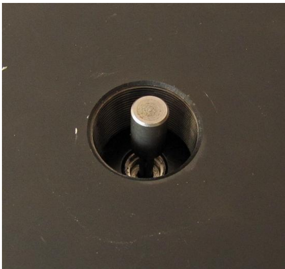
Placing “the puller” in the bearing casing
