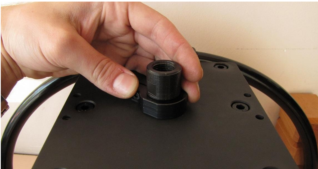
Affixing the clamping nut on the bottom cylinder
