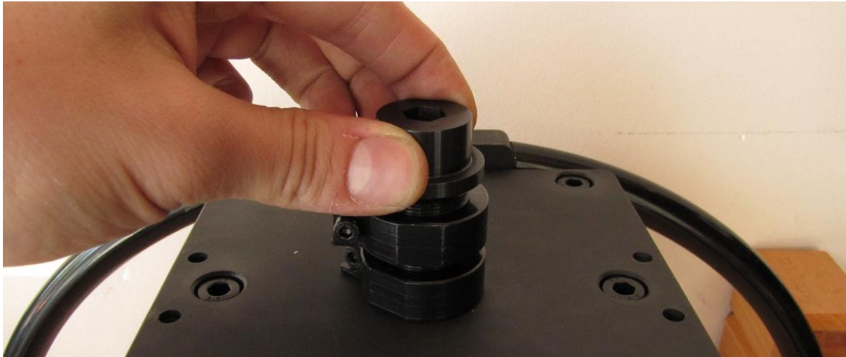
Screwing the spindle-pushing screw
