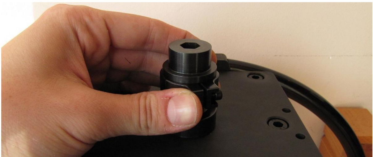
Marking the position of the bearing with clamping nut
