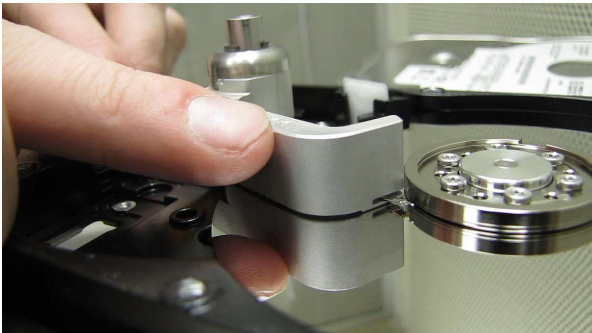
Picture 3. (lifting the heads)
