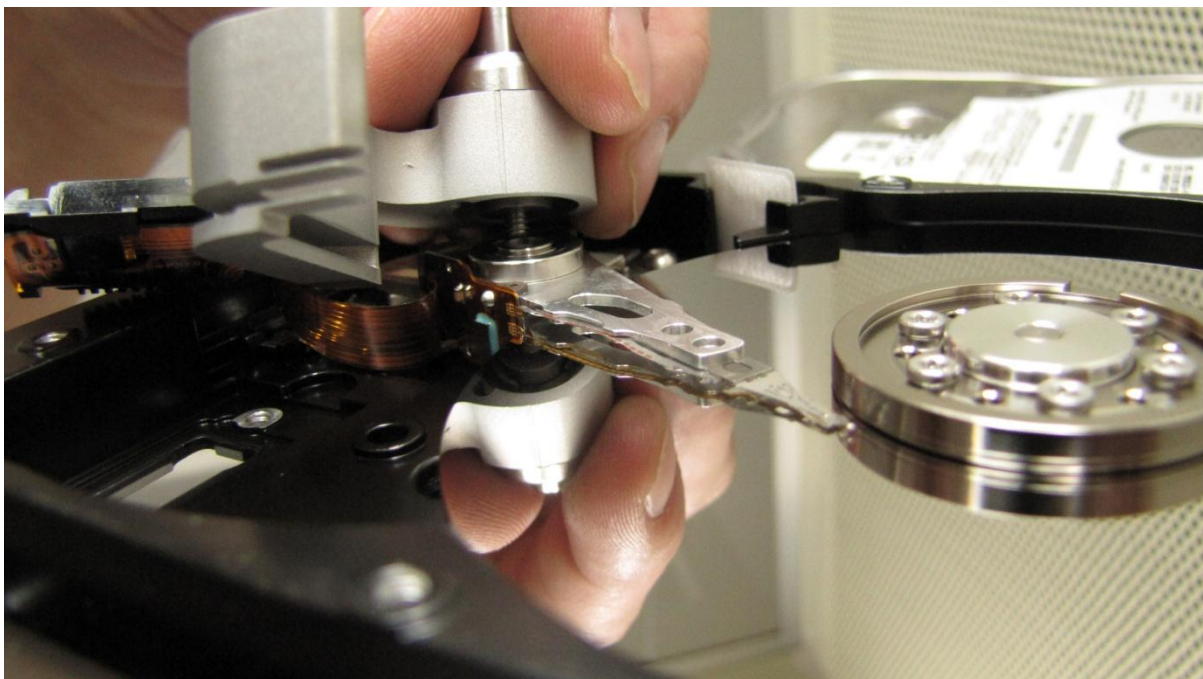
Picture 2. (mounting the tool)
