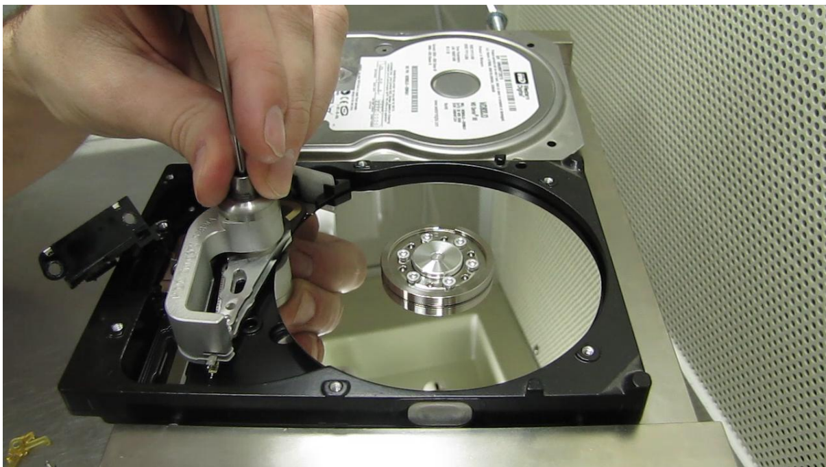
Picture 5. (unscrewing the head assembly)
