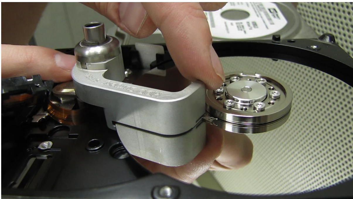
Picture 9. (returning the tool outside of platter)
