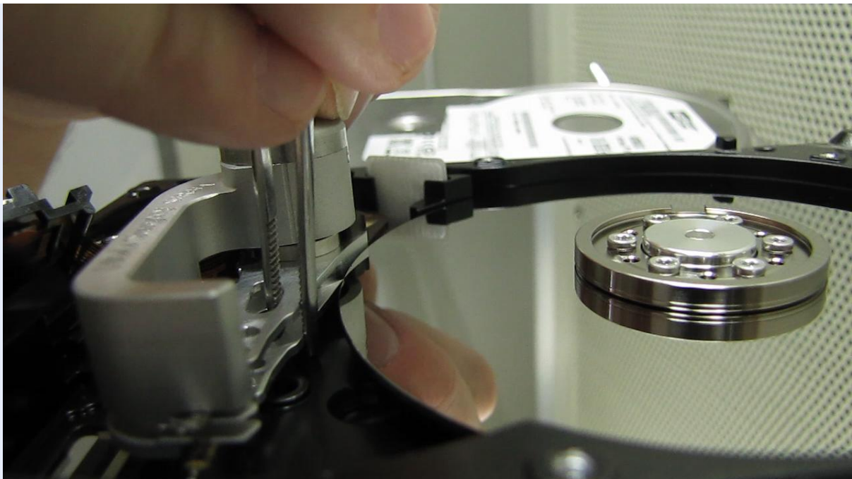
Picture 7. (mounting the heads on a patient drive)
