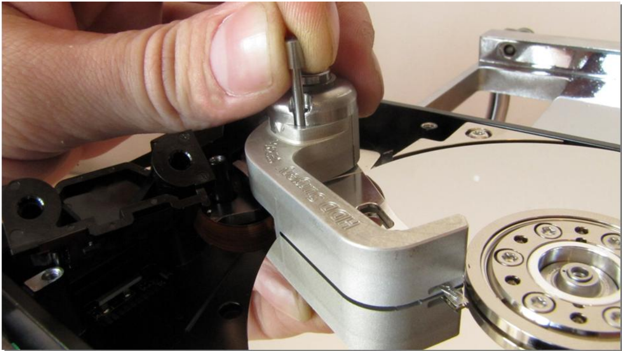
Picture 10. (remove the securing pin)
