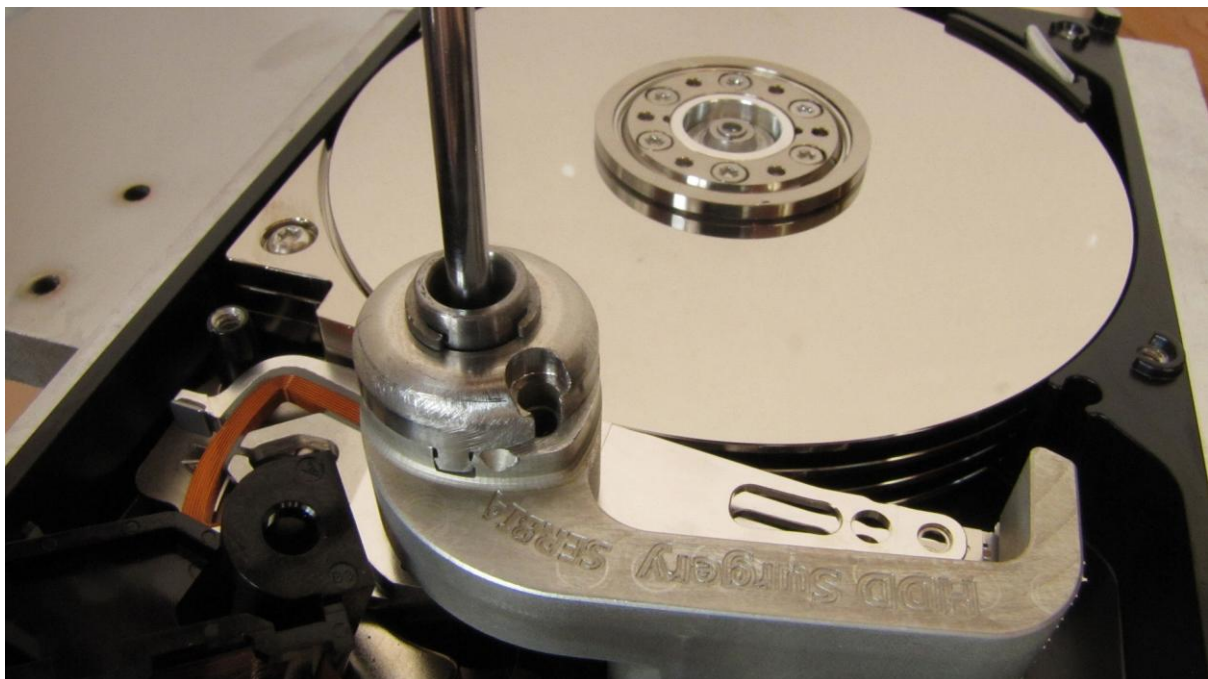
Picture 6. (unscrewing the head assembly)
