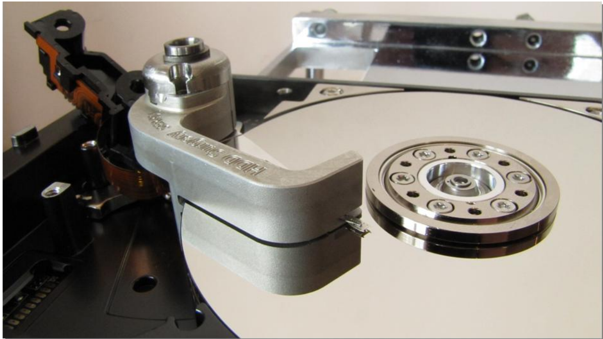
Picture 9. (moving the heads to their place)
