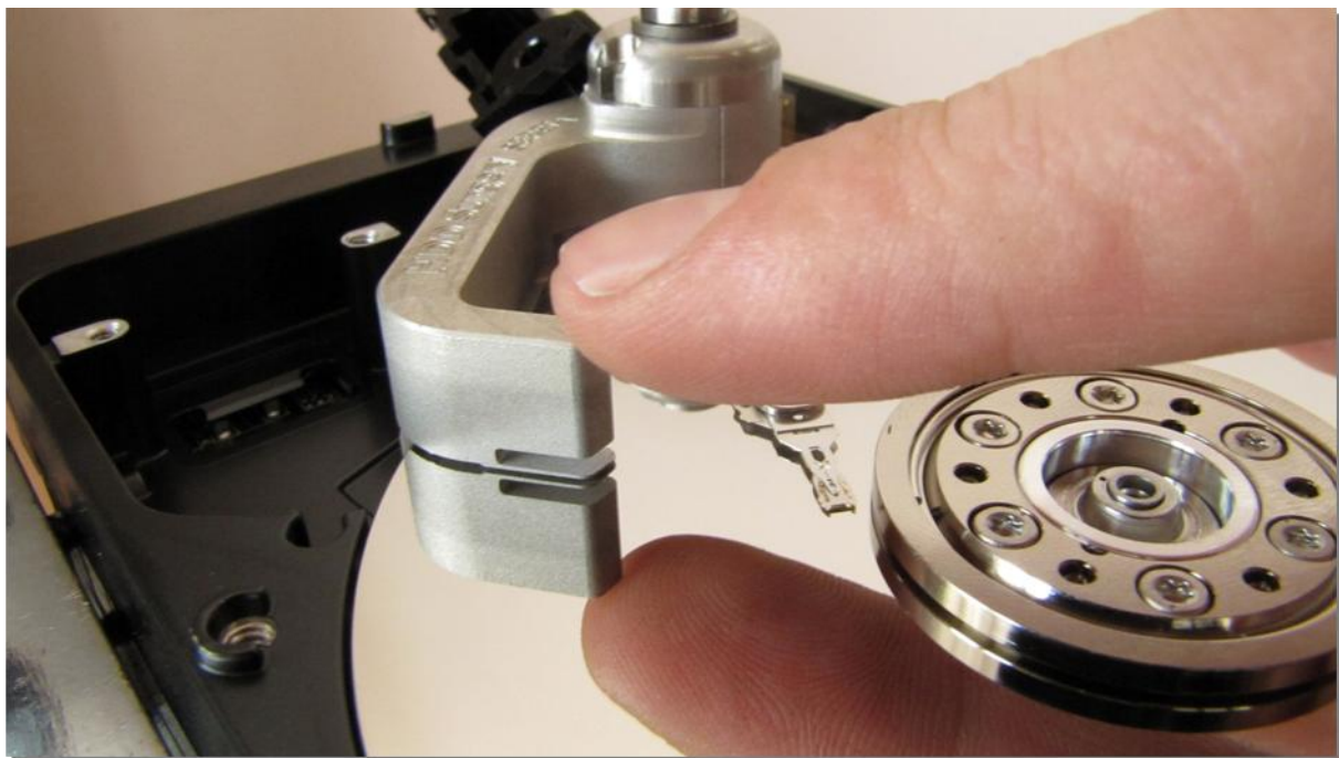
Picture 11. (returning the tool outside of platters)
