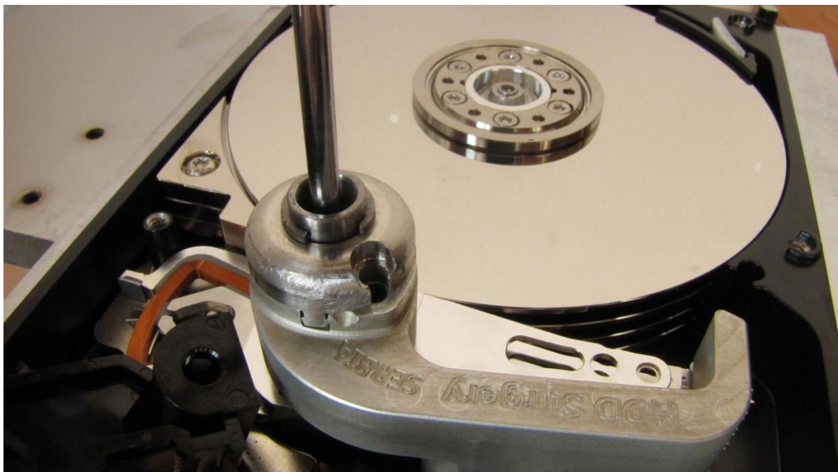
Picture 6. (unscrewing the head assembly)
