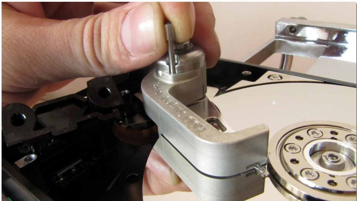
Picture 10. (remove the securing pin)
