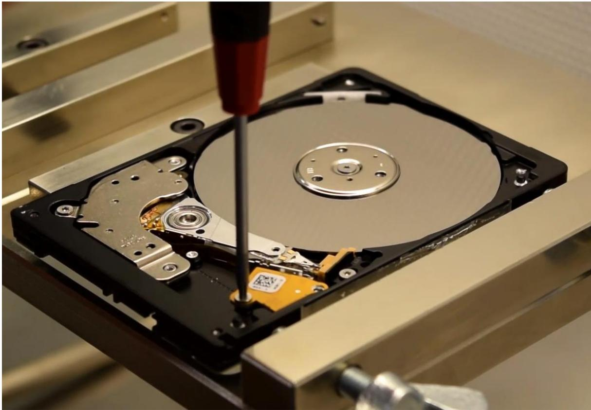
*Picture 5.3. Removing the flat cable*
