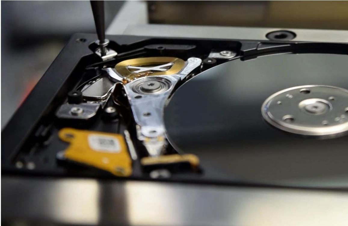
*Picture 5.6. Tightening the bottom magnet*
