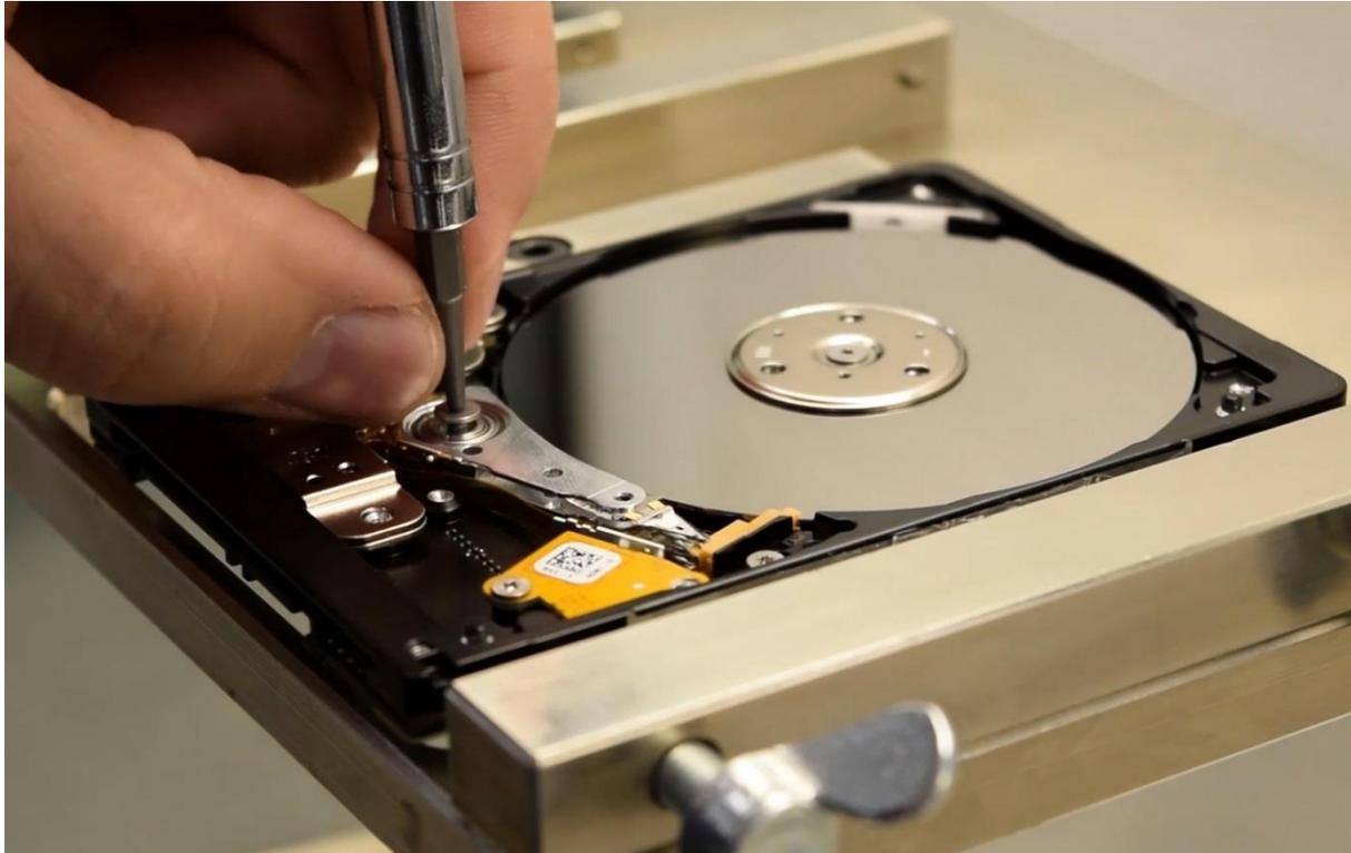
*Picture 5.18. Removing the screw from the HSA*
