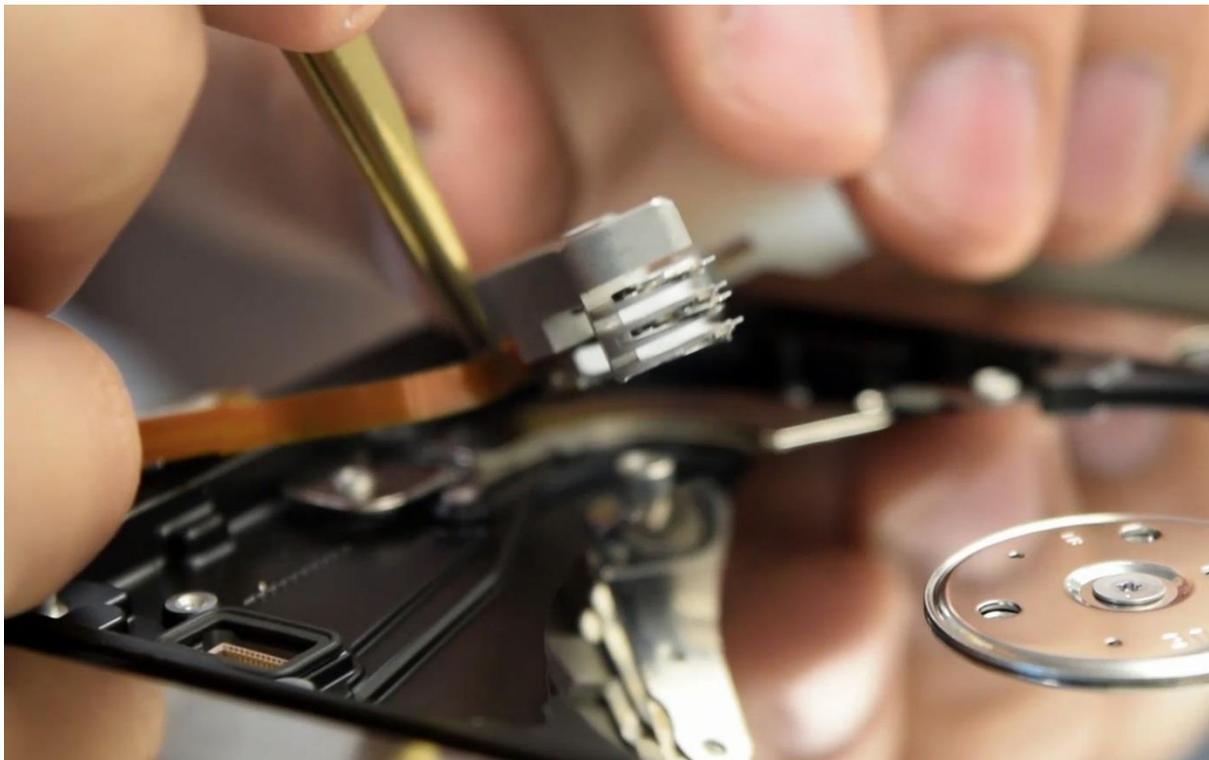
*Picture 5.12. Lifting the heads*
