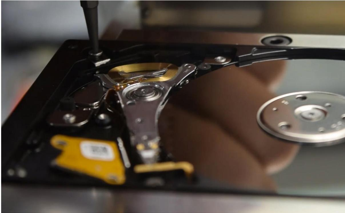
*Picture 5.17. Removing the screw from the bottom magnet*
