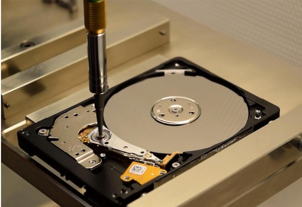
*Picture 5.4. Placing a bolt for securing the heads*
