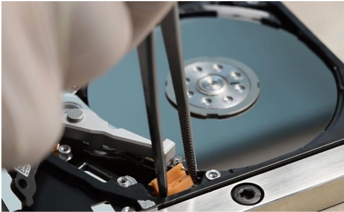
Picture 5.9. Dismounting the ramp
