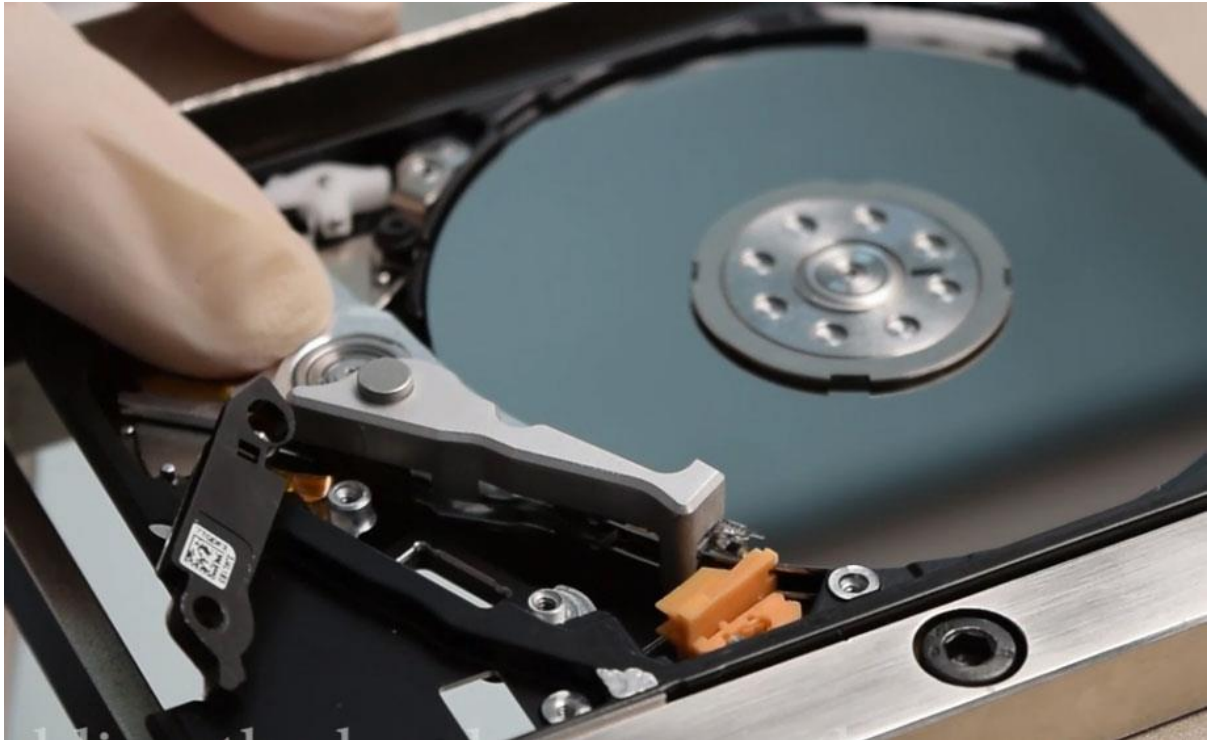
Picture 5.7. Moving the heads over the platters
