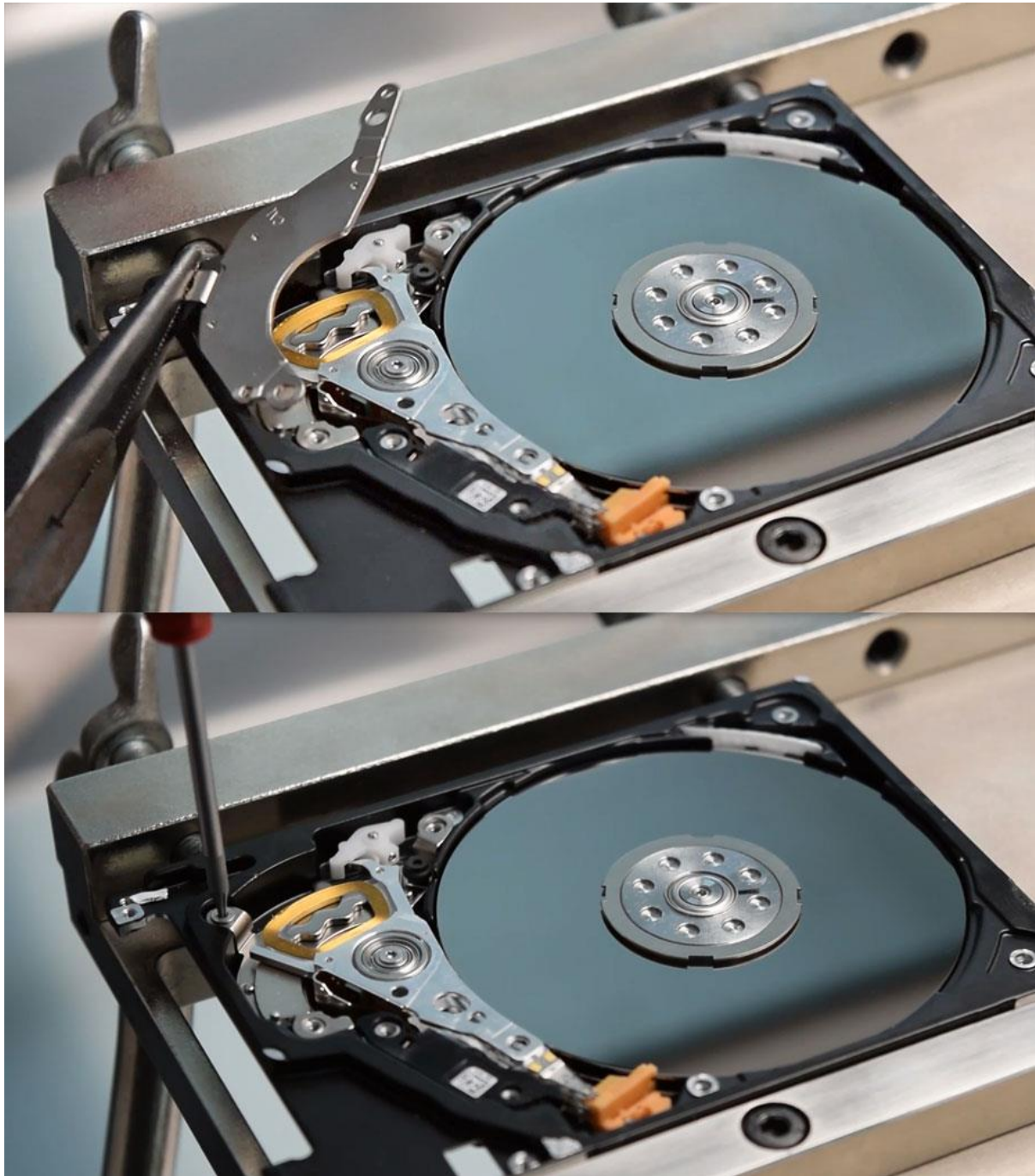
Picture 5.2. Removing the upper magnet
