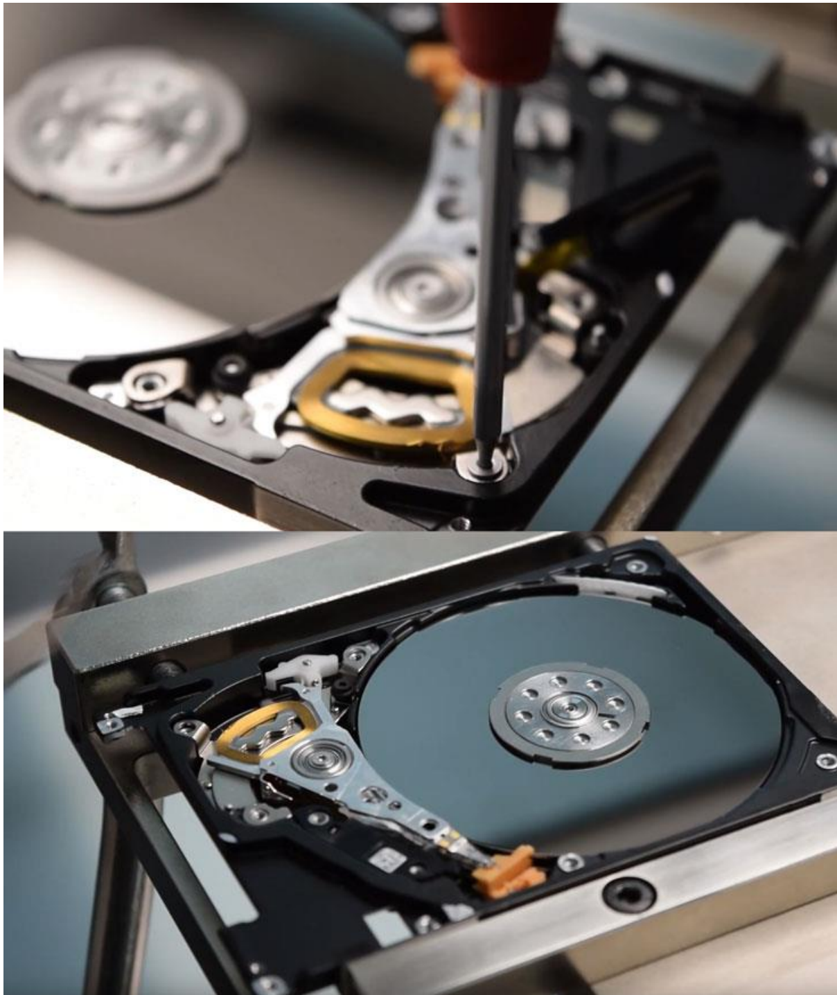
Picture 5.18. Removing the screw from the bottom magnet
