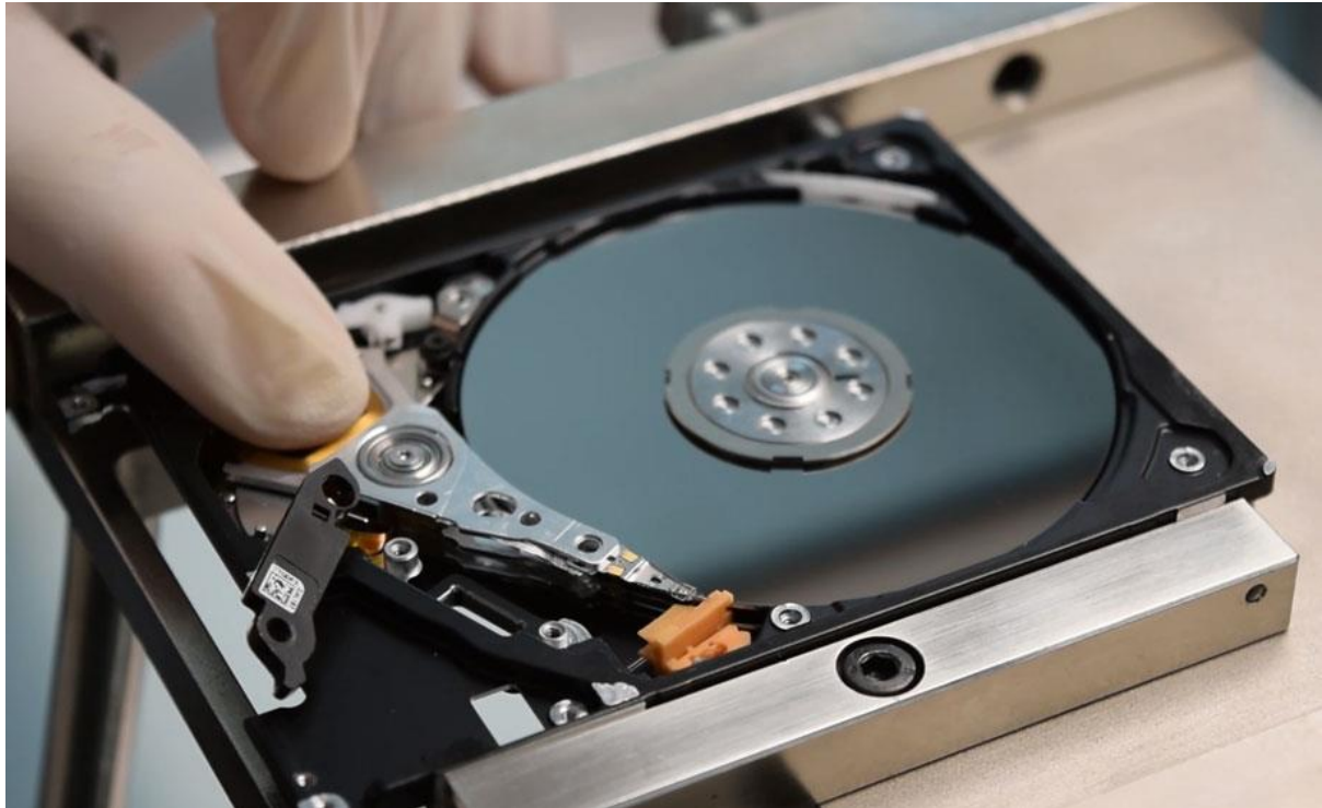
Picture 5.4. Moving the heads to the end of the ramp
