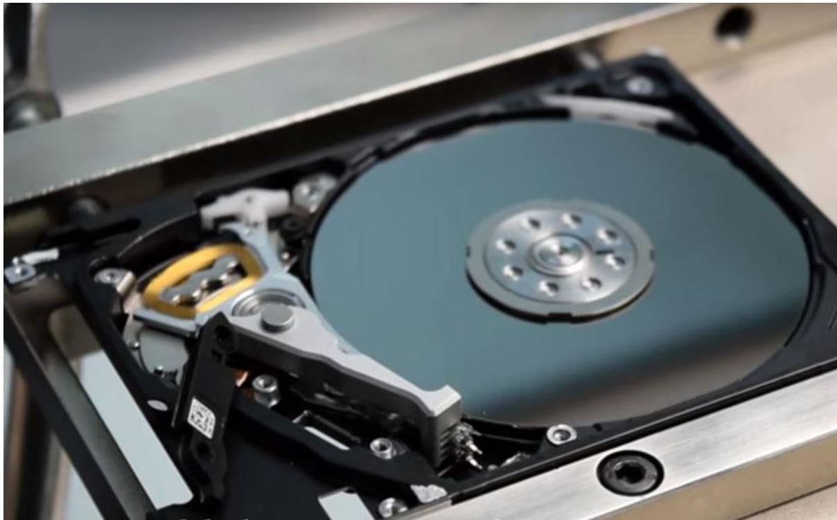
Picture 5.10. Sliding the heads off the platters
