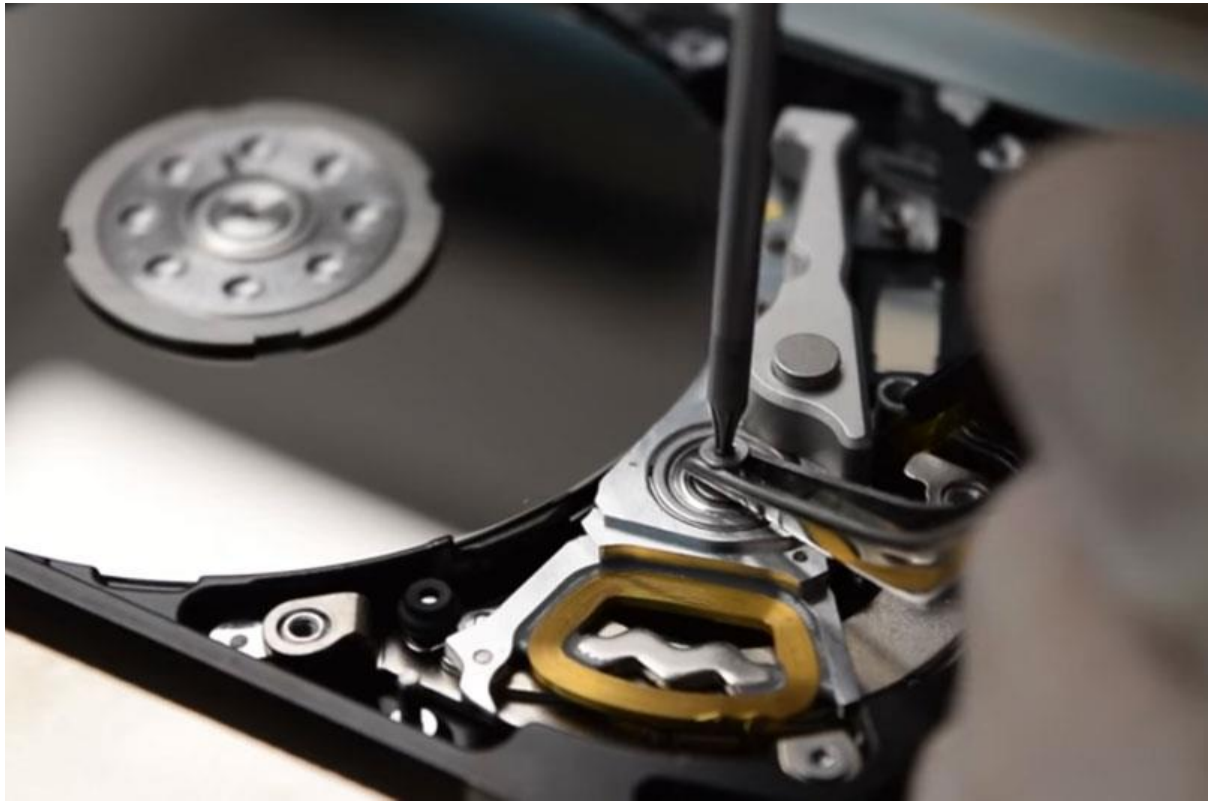
Picture 5.12. Removing the screw
