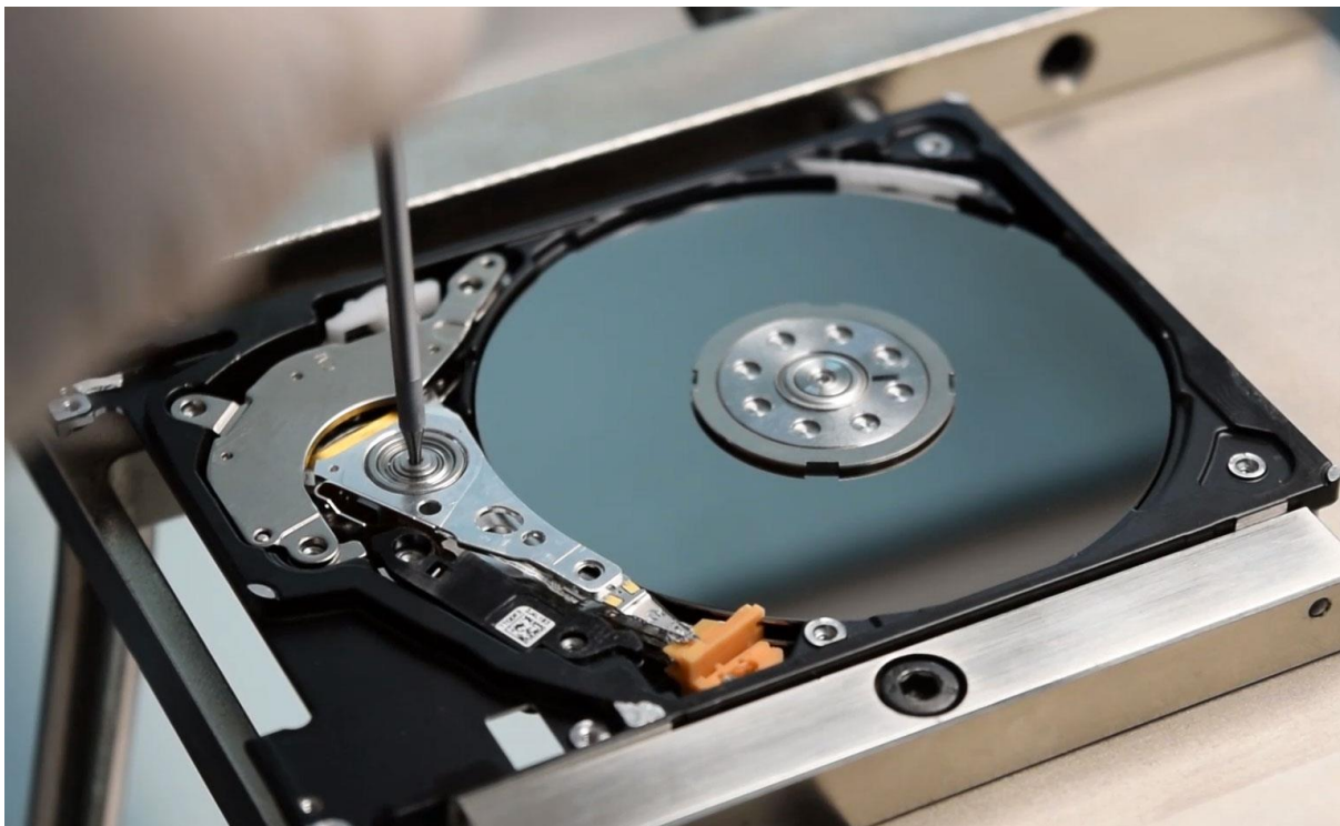
Picture 5.1. Inserting the bolt and securing the heads
