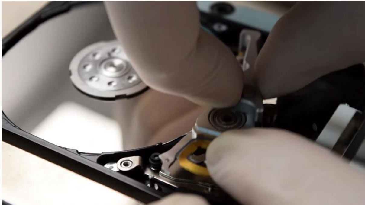
Picture 5.13. Lifting the heads
