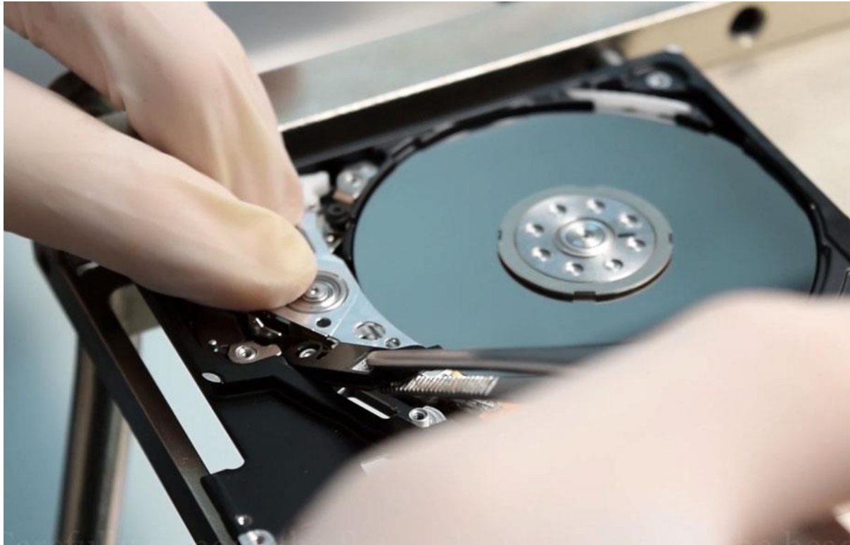
Picture 5.3. Removing the flat cable
