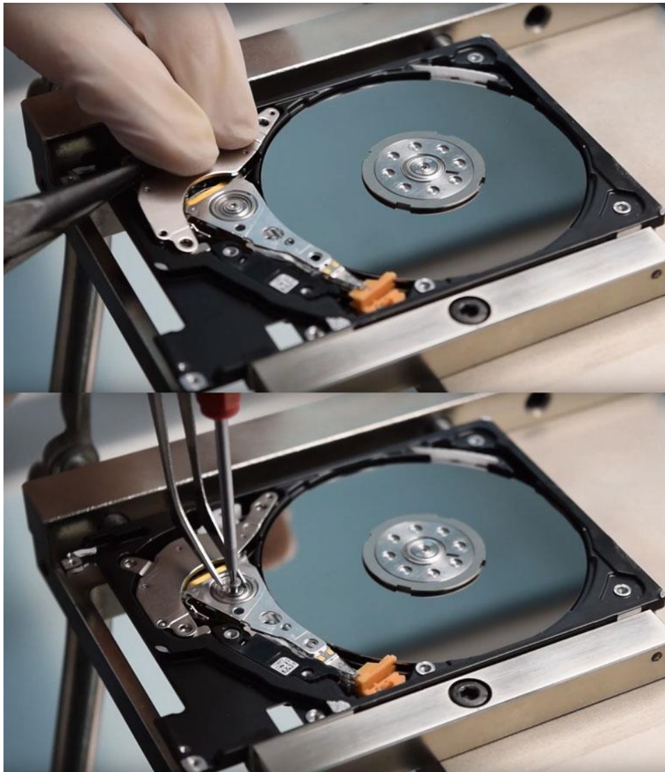
Picture 5.19. Removing the screw from the HSA
