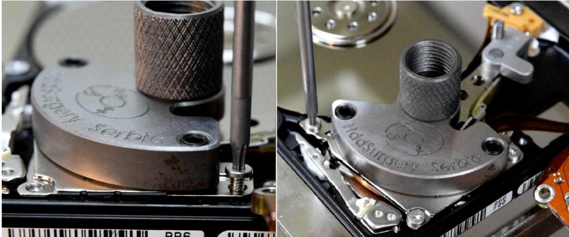
Picture 6.17 (Tightening three screws (fixing magnets to the patient drive casing))
