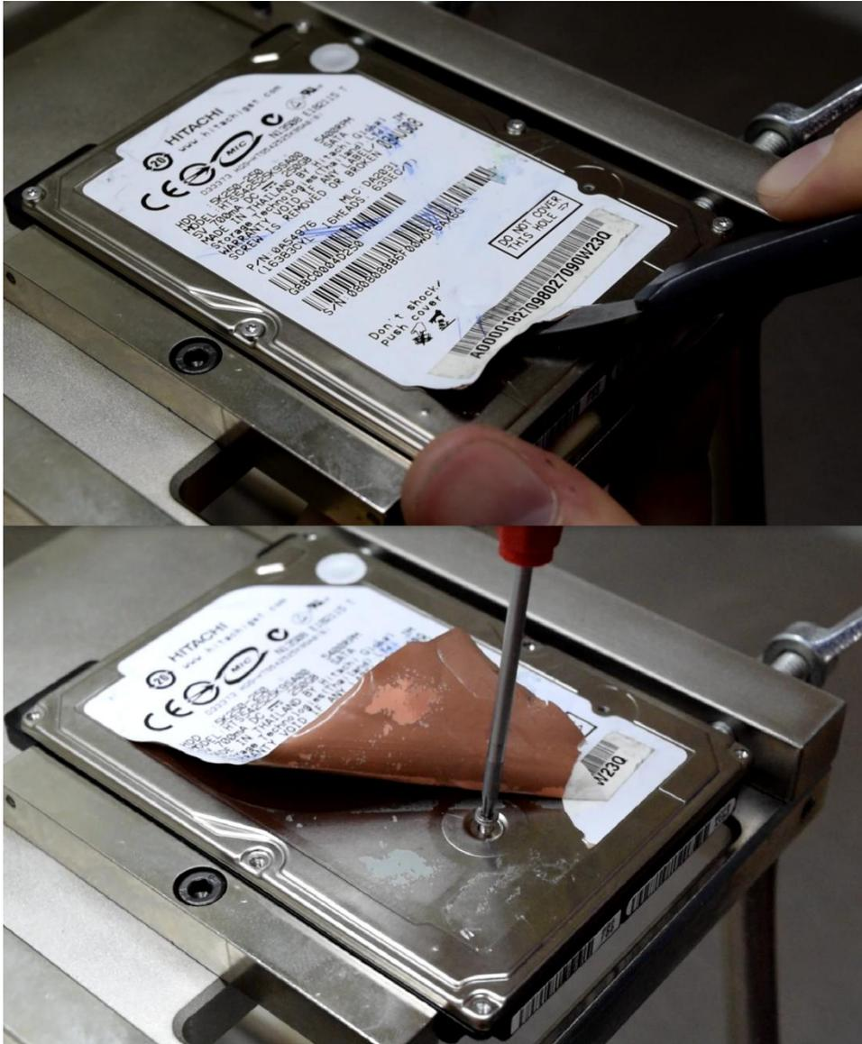
Picture 6.2 (Unsticking of the hard drive sticker (up) and unscrewing the lid (down))
