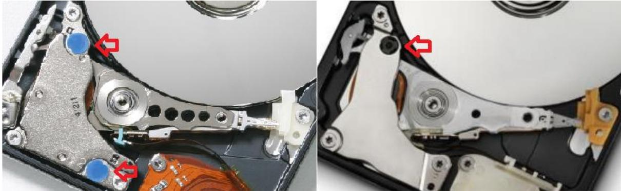
*Picture 4.2 (Left - Hitachi 2.5" hard drive with two security brakes on the upper magnet;
