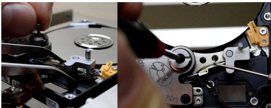
*Picture 6.10 (Inserting the screw into the threaded cocoon (left); tightening the screw which is connecting support tool and head assembly (right))*
