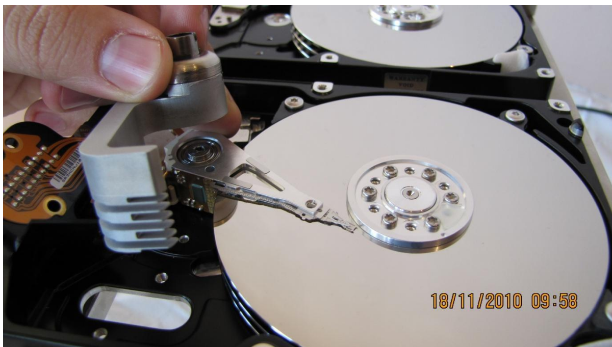
Picture 2. (mounting the tool )
